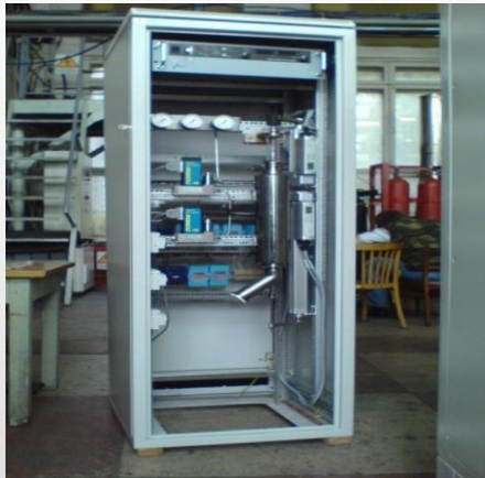
Installation for obtaining carbon nanomaterial capacity of 10 g / h
